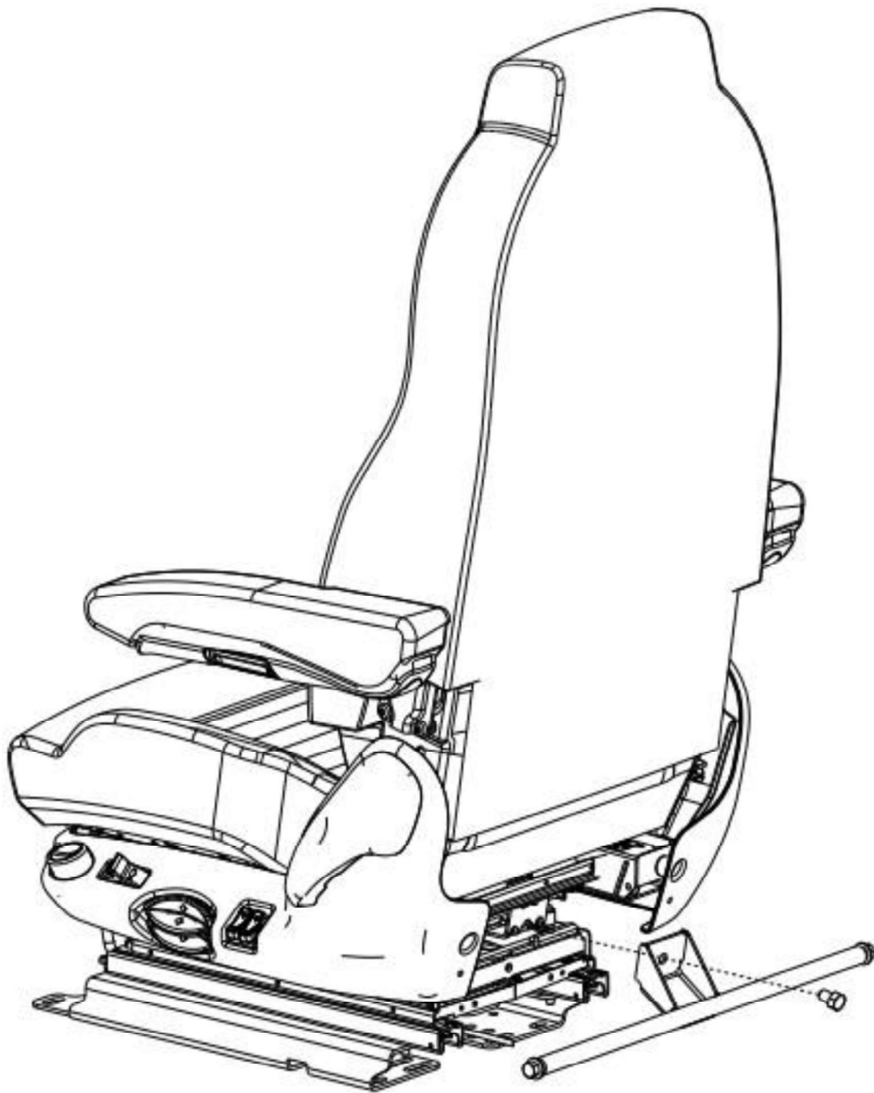
Figure #10: Regular Tether Installation
